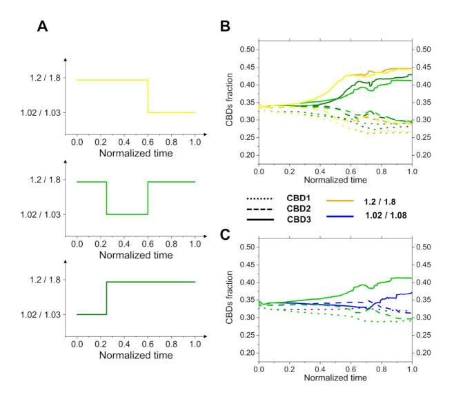
**Figure 6. A)** Schematic of the three-stage drying protocols implemented in this work, where the low DR rate step was applied at the end (yellow), middle (light green) and beginning (dark green) of the drying protocol. **B)** Comparison between the electrode fully dried at 1.2 / 1.8 and the ones dried with the three-stage drying protocols defined in A. **C)** Comparison of the less heterogeneous three-stage dried electrode and the one fully dried at 1.02 / 1.08.
