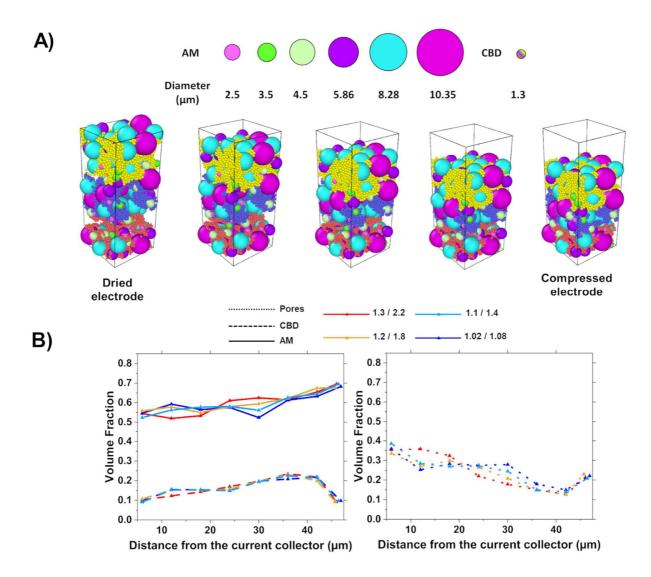
**Figure 4. A)** Evolution of the electrode mesostructures during calendering for the case of the electrode 1.3 / 2.2. The different colors (red, blue and yellow) of the CBD particles (indicating the 3 regions defined during drying, Figure 2) are kept just as a guideline for the eyes, but here all the CBD particles have the same physical properties. **B)** Evolution of AM and CBD (left) and bulk pores (right) volume fractions as a function of the electrode thickness.
