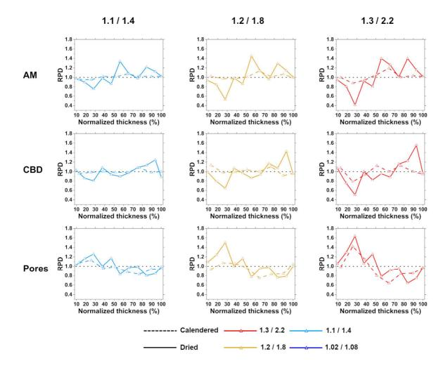
**Figure 5.** Evolution of the relative phase difference (RPD) for AM, CBD and (bulk) pore phases along their normalized thickness (0% stands for current collector side, 100% for separator side) for electrodes compressed (Calendered) or not (Dried) that were dried at different DRs. The black dotted line is a guideline for the eyes indicating an RPD equal to 1.
