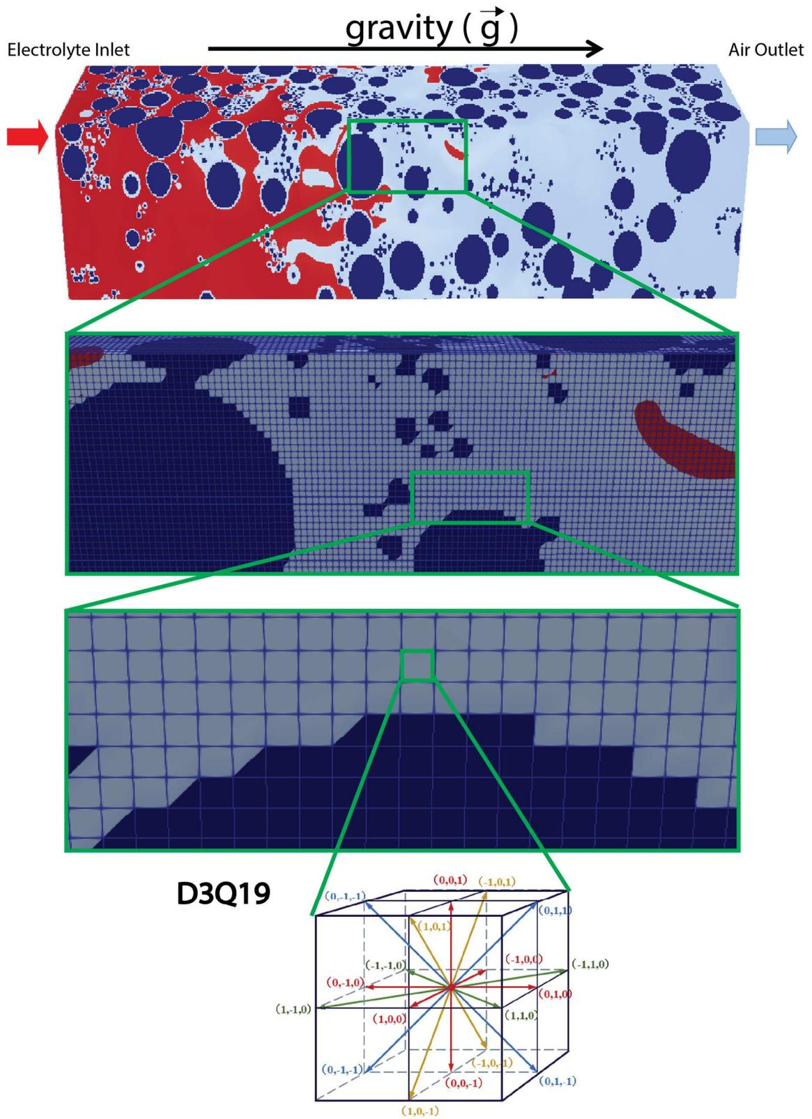
*Figure 2. Lattice structure of three-dimensional fifteen velocity (D3Q15) model.*
