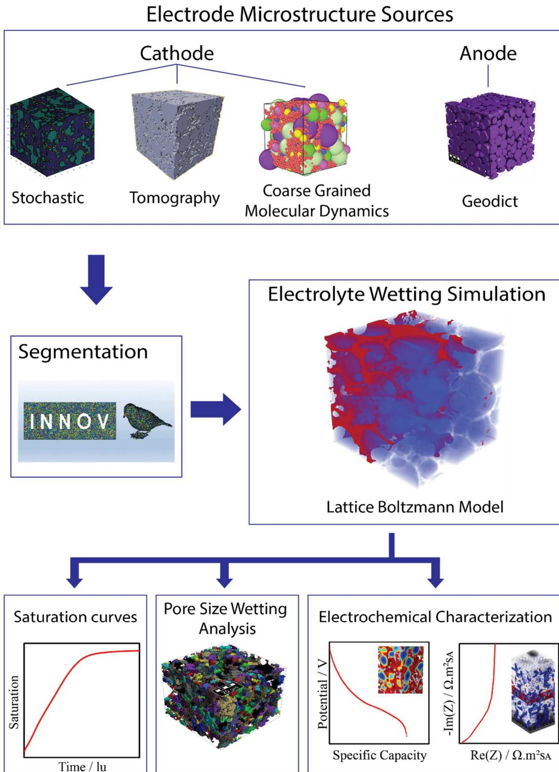
**Figure 1.** Schematic representation of the workflow used in the LBM simulation and its subsequent analysis.
