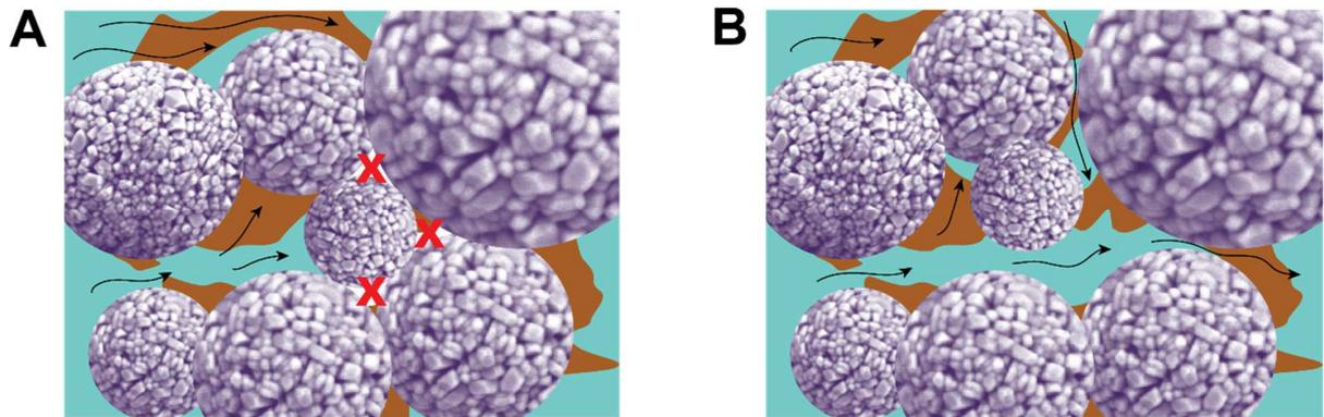
**Figure 9.** Schematics of ionic paths during the simulation of the electrochemical response (EIS or discharge) of the calendared tomography NMC 96% - CBD 4% electrodes for the case where the electrolyte does not fully fill the pores as calculated by the LBM for (A). *The case where electrolyte is assumed to fill all the pores of the electrode (B). Blue colour represents the electrolyte while brown colours represents the CBD.*
