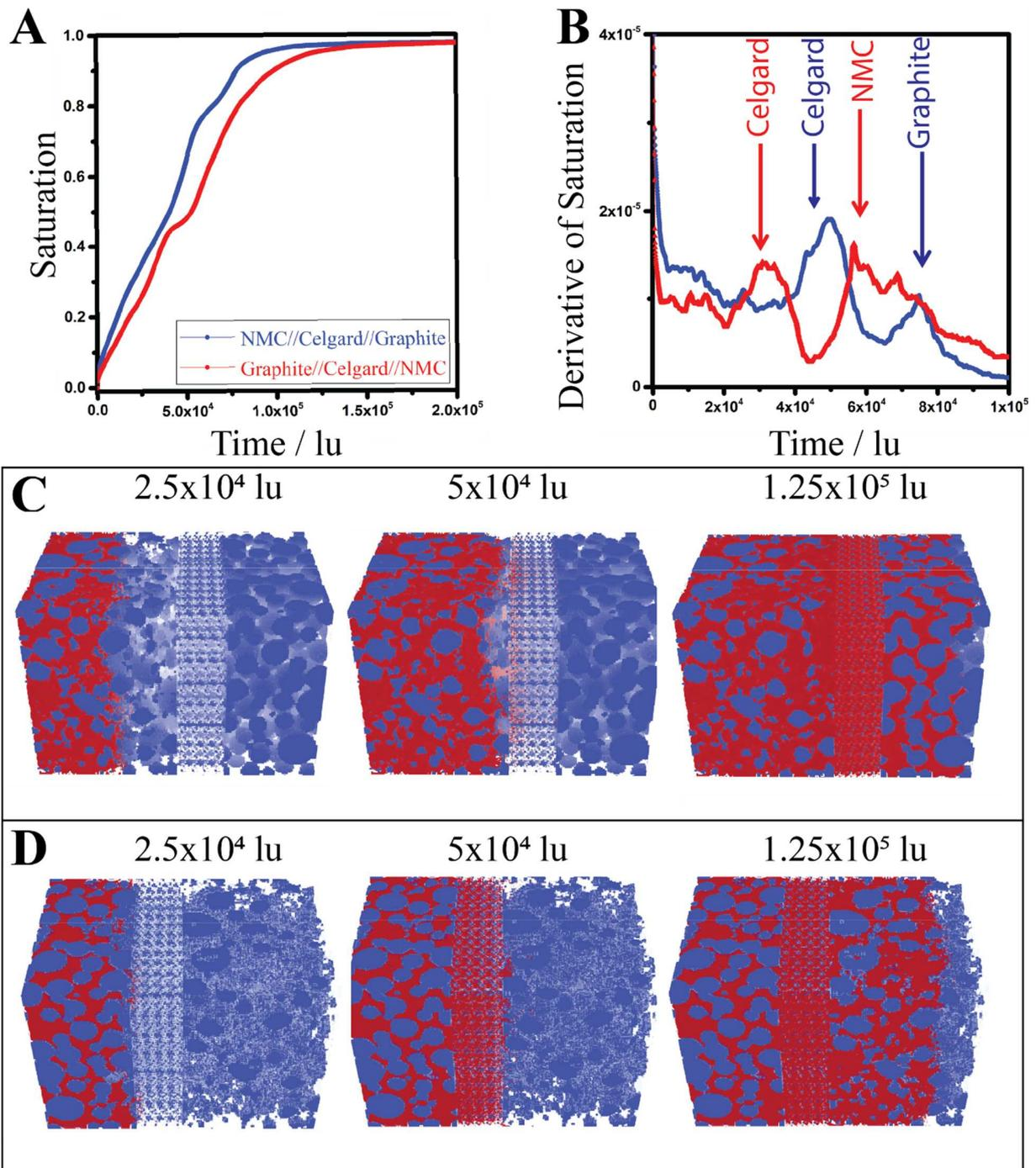
**Figure 7.** (A) Saturation curve for the NMC//Celgard//Graphite and Graphite//Celgard//NMC cells, (B) The first derivative of the saturation profile of liquid electrolyte in the cathode with various porosities, the wetting (red) process's visualization for the (C) NMC//Celgard//Graphite (blue) and (D) Graphite//Celgard//NMC (blue) at different time steps.
