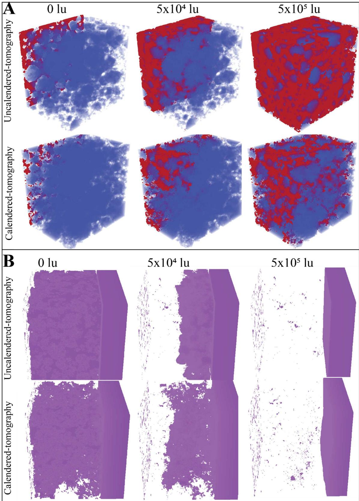
**Figure 5.** The wetting (red) process visualization for the (A) uncalendered and calendered tomography NMC 94% - CBD 6% (blue) at different time steps (B) the gaseous air (purple) in uncalendered and calendered tomography NMC 94% - CBD 6% electrode at different time steps.
