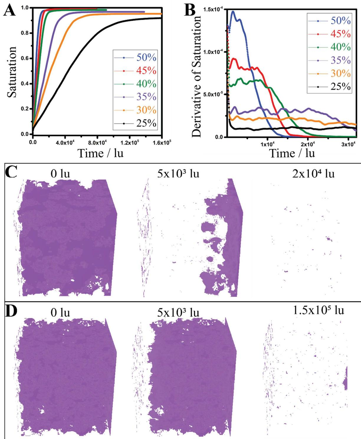
**Figure 3.** (A) Saturation profile of liquid electrolyte in the cathode with various porosities. (B) The first derivative of the saturation profile of liquid electrolyte in the cathode with various porosities. (C) The air output flow process (in purple) for the electrode with 50% porosity and (D) electrode with 25% porosity at different time steps.
