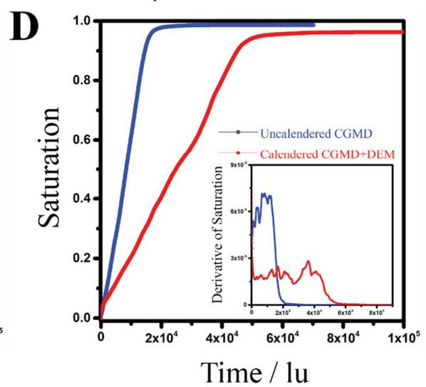
**Figure 4.** (A) Normalized pore size distribution for uncalendered and calendered tomography NMC 94% - CBD 6%. (B) Normalized pore size distribution for uncalendered and calendered CGMD+DEM. (C) Saturation profile and the first derivative (inset) of the saturation profile of liquid electrolyte for the calendered and uncalendered tomography NMC 94% - CBD 6% electrodes (D) Saturation profile and the first derivative (inset) of liquid electrolyte for the calendered CGMD+DEM and uncalendered CGMD.
