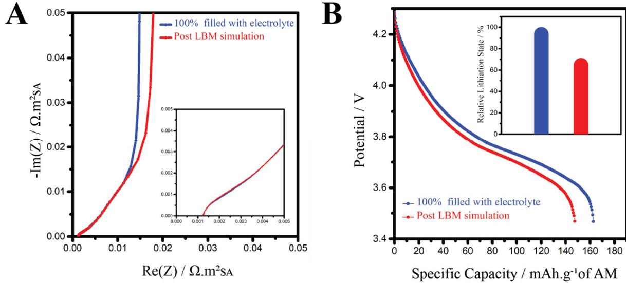
**Figure 8.** Simulated EIS and Discharge models for the calendared tomography NMC 96% - CBD 4% filled with 100% electrolyte and Post LBM simulated (A) Nyquist plots in the symmetric cell configuration, (B) Discharge curve at C/20 for the LBM output and the 100% filled electrode, the inset shows the average lithiation state of the AM surface in contact with the unfilled void at the end of discharge.
