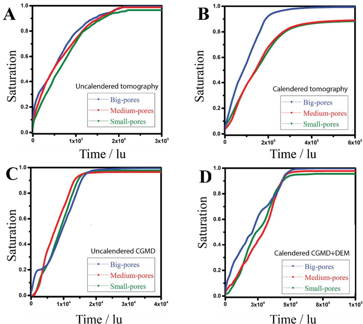
**Figure 6.** Saturation profile of liquid electrolyte three groups, big, medium, and small within (A) Uncalendered tomography NMC 94% - CBD 6% (B) Calendered tomography NMC 94% - CBD 6% (C) Uncalendered CGMD and (D) Calendered CGMD+DEM
