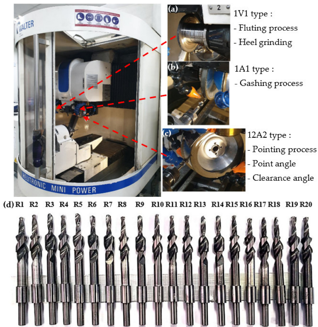
Figure 2. Location of grinding wheel for the tool fabrication (a) fluting wheel, (b) gashing wheel, (c) clearance/point angle wheel, (d) finished drill with customised geometry of twist drill types.
