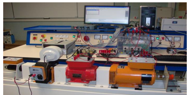
Fig. 20 The experimental system in the L.T.I laboratory (University of Picardie, I.U.T of AISNE, 02880 CUFFIES) consisting of a 1.5kW induction motor, a voltage-source inverter, and a digital signal processor (DSP).
