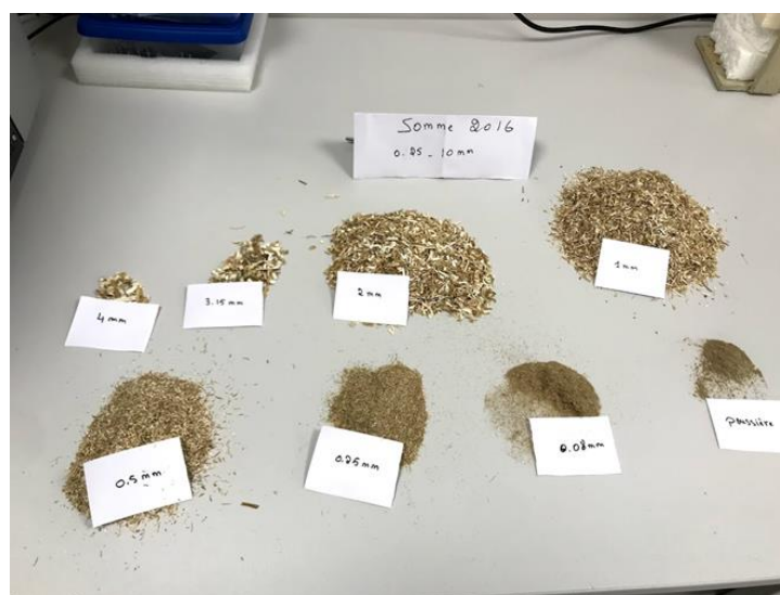
Figure 3. The different sizes of rapeseed straw after the sieving test.
