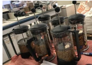
Figure 4. Experimental method for measuring water absorption.
