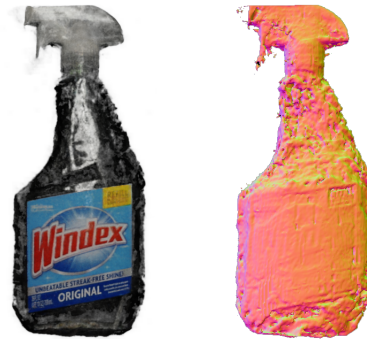
Fig. 2. Windex rendering and geometry with white rendering background (and black scanning background) shows how scanning background color is assigned to transparent surfaces.
