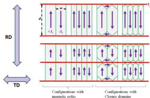
Fig. 6 : Line spacing  $d$  definition and impact.
