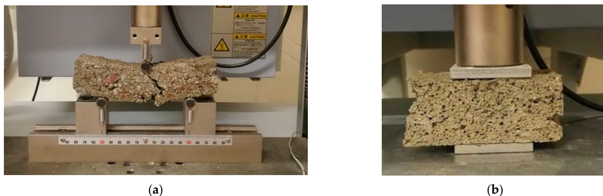
Figure 4. Flexural (a) and compressive (b) strength tests carried out on one of the biopolymer composites.
