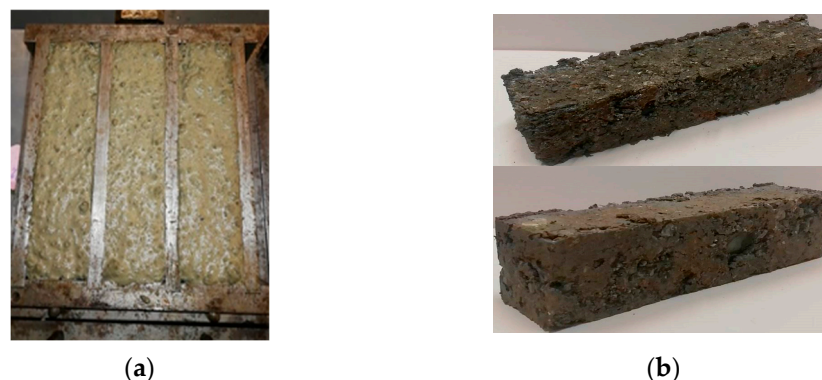
Figure 3. Photographs of (4 \times 4 \times 16) cm 3 test species: (a) mixture poured in molds and (b) full test specimens.
