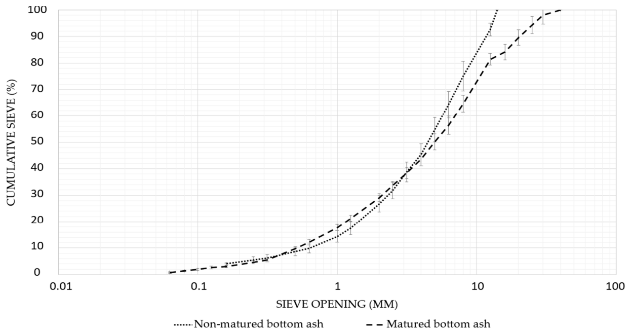
Figure 6. Particle size analysis of bottom ash samples.
