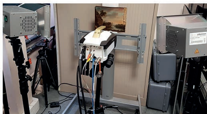
IR Camera 7.5-11.5 μm, 50 mm with ring 0.25", L_c = 0.55 \text{ m} , L_r = 0.8 \text{ m} , E(f) = 3 \text{ kJ (9)} , \nu(\text{Hz}) – the Fourier frequency, Image in Phase Shifts or Amplitude.
